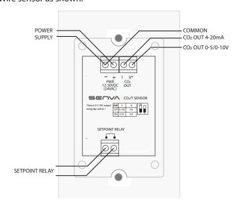
3. Set DIP switch positions to accommodate your application. DIP switch 2 only applies to units with transmitter temperature output selected.
